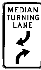
Median turning lane sign
