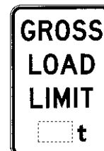
Gross load limit sign
